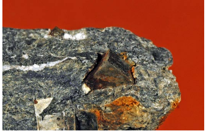
Pyrite with thin goethite coating, near Sulzer, Prince of Wales Island, Alaska; crystal is 5 mm across.
