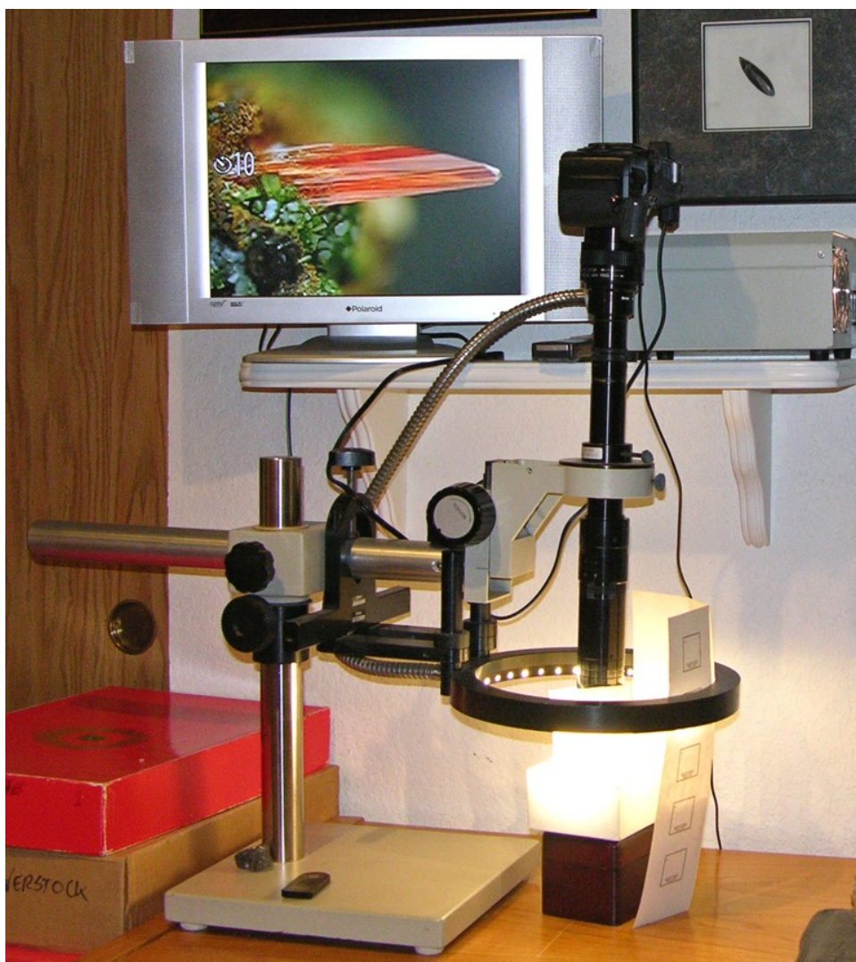
Figure three: One Type of Photomicrographic Set-Up, this one centered around an Optem Zoom 125C machine vision lens.
