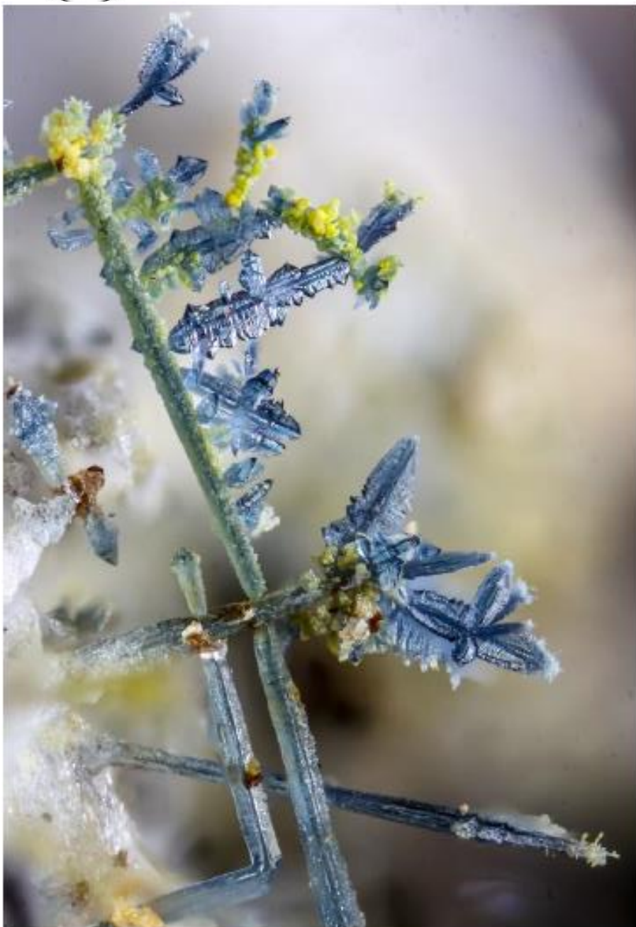
Cassiterite and minor varlamoffite Genna Zinc Smelter. FOV 2.0mm
