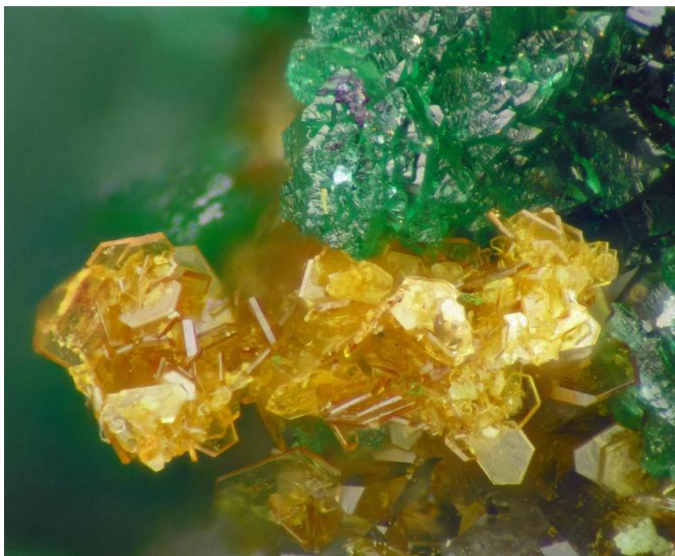
Unknown Orange-Brown plates on Malachite—Centennial Eureka Mine— 1.2 mm. EDS and WDS analysis revealed Pb, Fe, K, & As with a trace of S and Ti, zoned with some low Pb areas. This composition matches no known mineral species. The crystals appear to be tabular on {0001},
