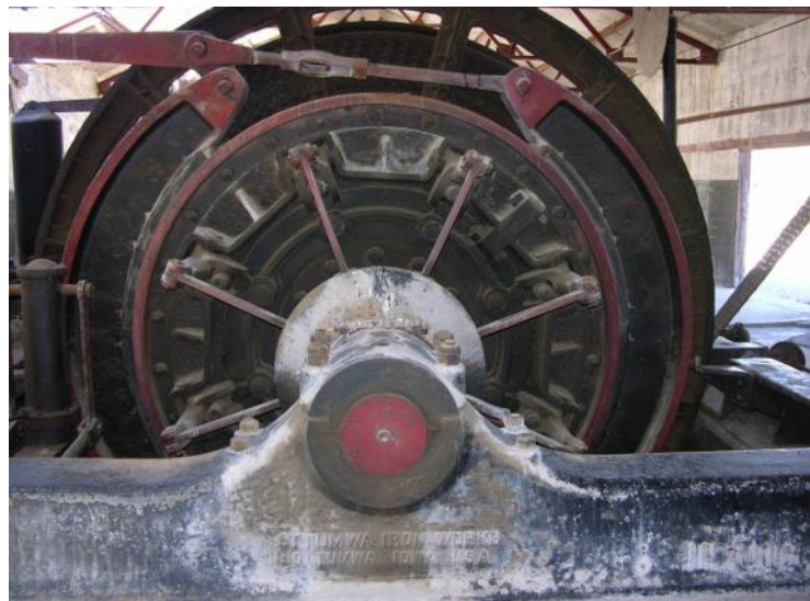
Huge Pillow Block that holds the Hoist Assembly at the Eagle and Blue Bell Mine.
