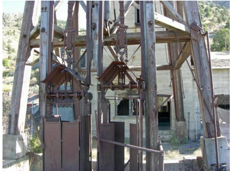
Man-Lifts Suspended Over the Shaft at the Eagle and Blue Bell Mine— note the hand woven belts above the lifts.
